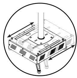
**Step 2.** Once the screws have been loosened, slide the GB-PIPE1 laterally side to side (or front to back).
